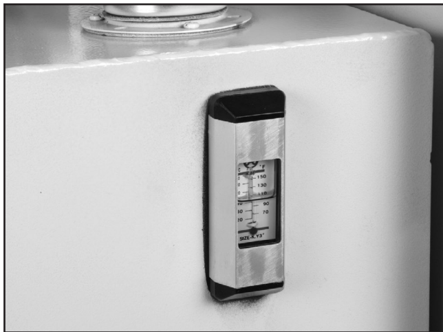
Figure 53. Hydraulic fluid reservoir sight glass (rear access panel removed for photo clarity).
